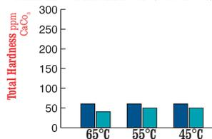
The total hardness test is described in “Water Conditioning for Industry” by S T Powell pages 476-479 (McGraw - Hill 1954 source Mr R Gregory, WRc). Three water samples (hard, moderately hard and soft) were used and heated to three temperatures (65°C, 55°C and 45°C).
